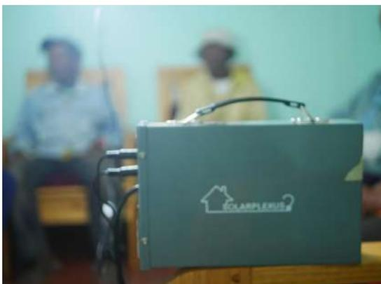
Once the battery recharged and brought back to the user's home, the lighting kit can be connected to the battery to benefit from a quality lighting > 1500 lumens, and this, 7 hours / day during 3 days in a row.
